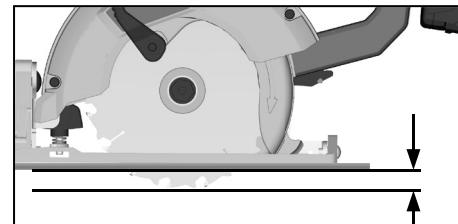
Adjust the cutting depth to the thickness of the workpiece. Less than a full tooth of the blade teeth should be visible below the workpiece.
