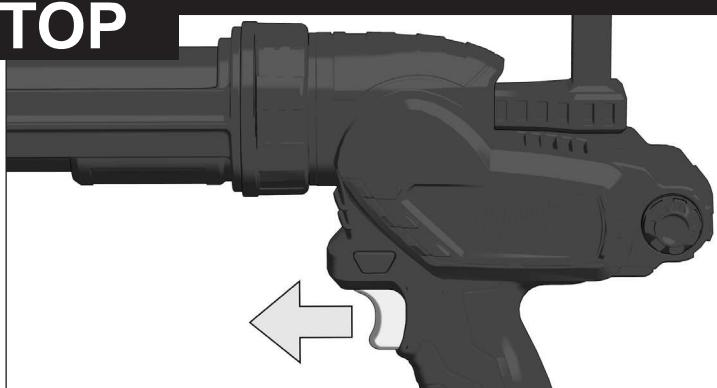
When the trigger is released, the motor will run for a short time to release the rod. This prevents a drip.
